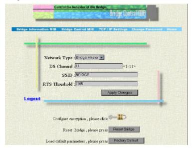
Network Type – Set the serving type of Bridge. This field can be set to "Access Point"
