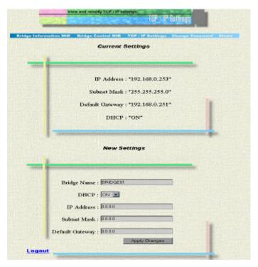
NOTE: WL11000SA-N (B) build in the DHCP Client function, it means the Wireless Bridge will get the IP address, subnet mask and default gateway values from DHCP server while Wireless Bridge powers on the network.
